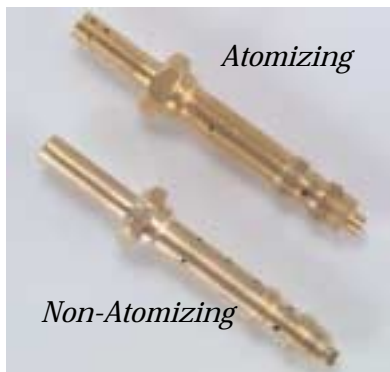
Left: Brass discharge nozzles. Top nozzle is of the pepper-box design. This atomizing design is frequently installed in the smaller TCM carbs to correct erratic fuel flows associated with the installation of the single-piece venturi (Precision S.B.s MSA-7, MSA-8, MSA9).
