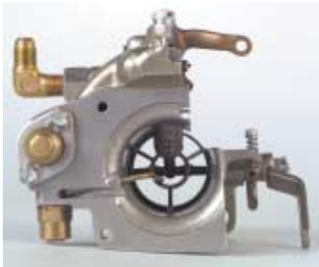
Looking up the throat of the MA-4SPA Carburetor. This vantage point reveals the proper placement of the pump discharge tube. The tube must be positioned just within the center ring of the primary venturi.
