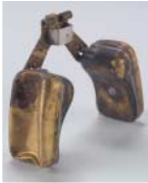
Photo shows a collapsed brass float. Never introduce shop air to the inlet fitting, discharge nozzle, or fly holes in the throat of the carburetor — the high pressure might collapse the float.
