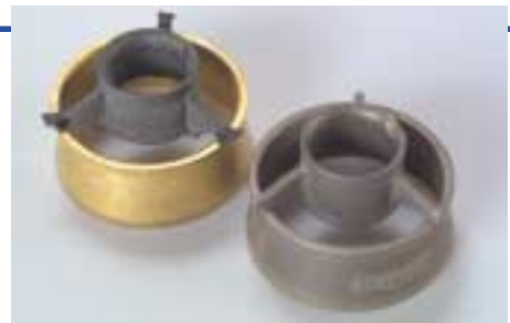
Venturis. The two-piece venturi (above left), is subject to annual and 100-hr inspections as per AD 98-01-06. Single piece venturi (above right) requires no recurrent inspections. Carburetor data tags with 'V' stamped on them indicate that the single piece venturi has been installed.
