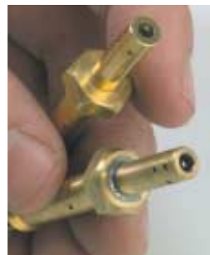
Right: Kelly Aerospace Power Systems manufactures discharge nozzles from a single piece of stock (top). Older discharge nozzles are welded where the neck meets the wrenching flats. Heavy porosity or a side load on the neck may compromise these welds. Visually inspect the integrity of the nozzles to assure that the neck will not separate from the body. The neck of the nozzle would be ingested into the engine if such a separation occurred.
